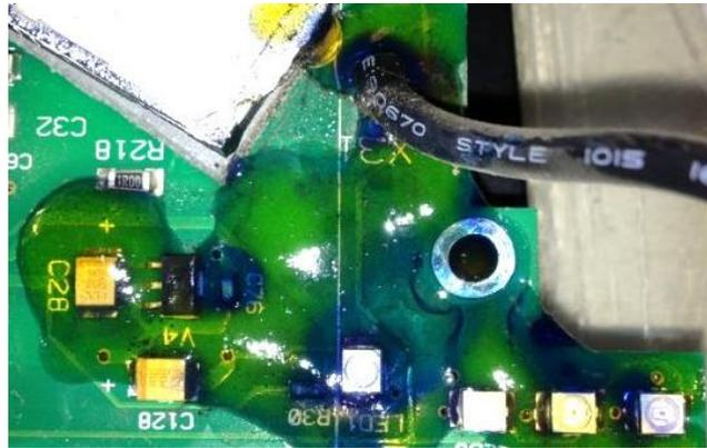
Figure 3: Corrosion induced by hygroscopic dust particles in the user environment
