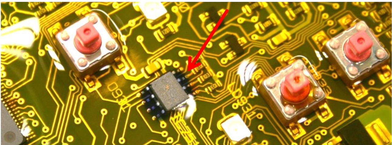
Figure 2: Reflow flux residue induced corrosion
