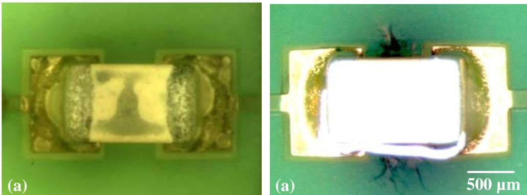
Figure 1: (a) Corrosion on the SMCs (after exposure to high humidity), and (b) corrosion under the SMC (after exposure to humid conditions, corrosion is induced by reflow flux residues)
