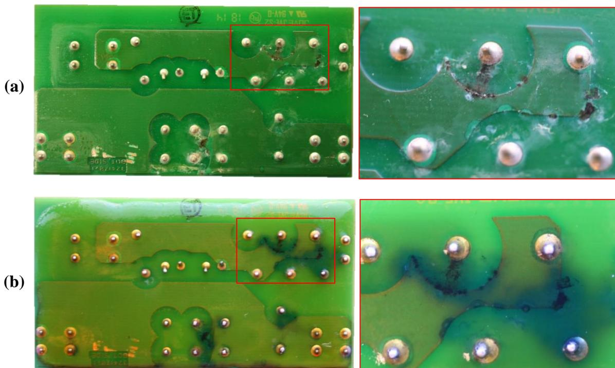
Figure 4: Tin corrosion under AC voltage (PCBA from the field return): (a) before and (b) after application of the gel
